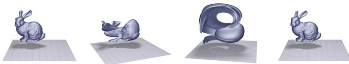
Fig. 8. Extreme level set deformation of a high-resolution model exhibiting very thin walls. The Stanford bunny is advected by a divergence-free and periodic vector field [LeVeque 1996; Enright et al. 2002]. The maximum bounding grid is 1024^3 , but memory requirements never exceed 97 MB. From left to right the simulation times are (in units of the period) 0, 1/15 , 1/2 , 1.
