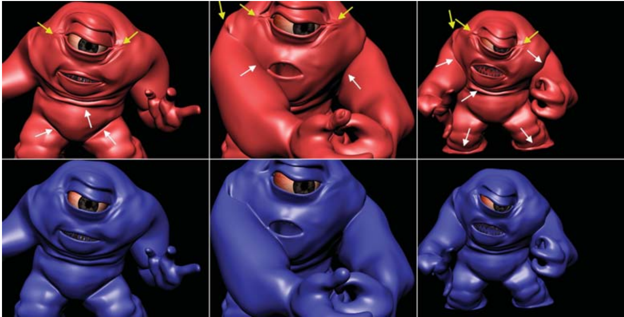
Fig. 5. A demonstration of our robust scan conversion algorithm described in Section 6.2. Top: The original Tar Monster character mesh (red) was often ill-posed. The white arrows denote regions of self-intersections. The yellow arrows point at crevasses or sharp ridges. Bottom: The RLE level sets (blue) resulting from the scan conversion of the Tar Monster 's 69,120 faces and 69,153 vertices. The original conversion, at a resolution of 624 \times 554 \times 488 , was able to resolve the mesh and its regions of self-intersections into a closed level set. The subsequent down-sampling, to a resolution of 312 \times 277 \times 244 , reduced the temporal aliasing artifacts caused by the original mesh's moving sharp ridges and crevasses. The whole process of scan conversion, down-sampling, and subsequent rendering took an average of 7 min/frame.
