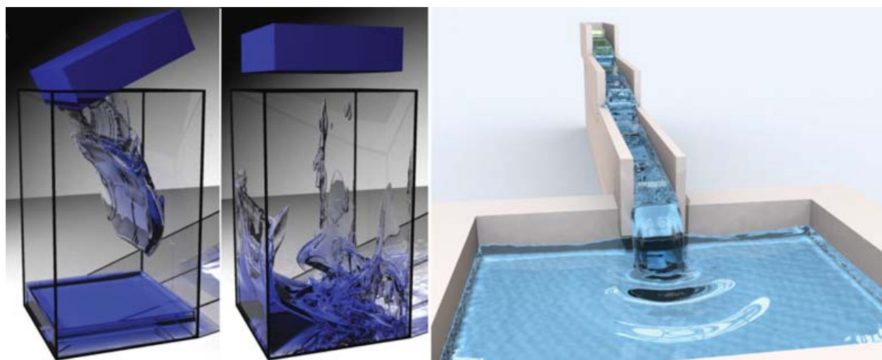
Fig. 11. Two fluid simulations using RLE level sets to achieve a large simulation bounding volume without incurring a similarly large memory burden. Left: The bounding volume is 136 \times 136 \times 320 (6 million voxels) while the memory usage is only 20 MB, 77% less than the 90 MB of memory required by a corresponding dense field fluid simulation. Right: The bounding volume is 444 \times 178 \times 102 (8 million voxels) while memory usage is only 30 MB, 75% less than the 130 MB of memory required by a corresponding dense field fluid simulation. See Section 6.6 for details.
